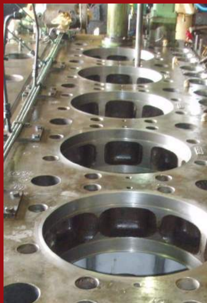
Machining 6 cylinders + positioning inserts in ten days.
