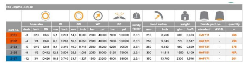
WJTA-IMCA Color Coding Scheme for Pressure Hoses - Maximum Working Pressure Applicable
